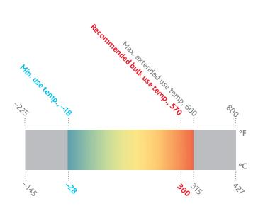
Eastman Therminol<sup>®</sup> 55 heat transfer fluid is a unique, synthetic fluid designed to provide reliable, consistent heat transfer performance over a long life at recommended bulk temperatures up to 300°C (570°F).
